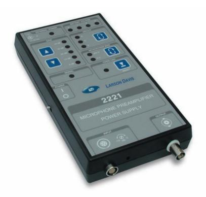
The Model 2221 is an excellent choice for when you need a traditional preamplifier power supply. The Model 2221 includes all the features needed for demanding applications such as low noise amplification and the ability to drive long cables up to 500 feet. It includes built-in A, C and Z weighting filters and can be powered from internal AA batteries or an external AC adapter.
